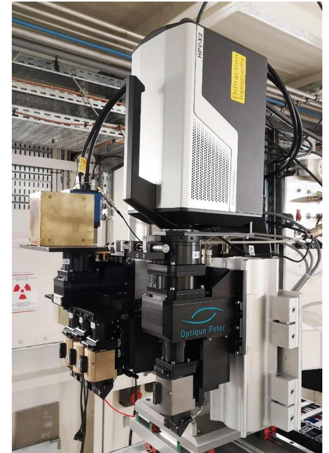
NUV White Beam Single objective microscope 1 Million i/s with Shimadzu HPV-X camera ESRF-ID19
