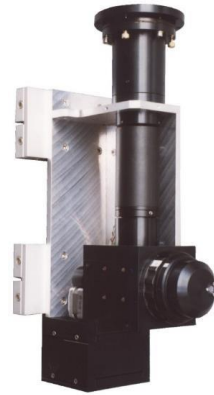
First Monochromatic Beam microscope delivered to ESRF / ID22 in 1997
