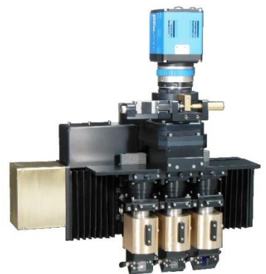
White Beam 3 objectives/ 3 scintillators
